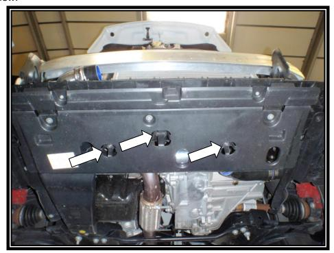
21. Position the hard pipe so that the slotted brackets are in line with the threaded holes. Please insure that hose 1368 is fitted in a position so that it is clear of the radiator. The bottom part of under tray has been dropped down only for visual reference on boost pipe position.
