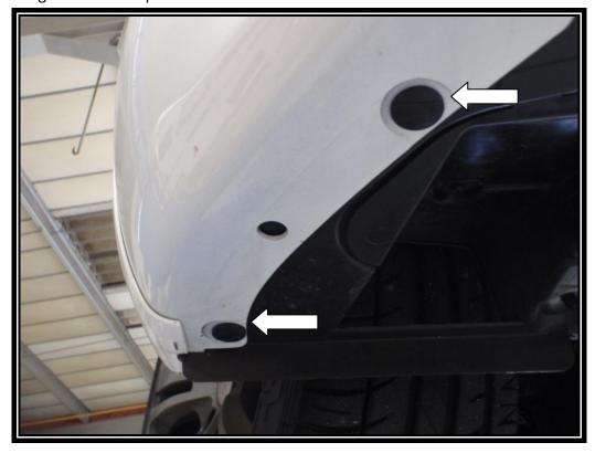
3. Undo the two bolts under the front bumper
